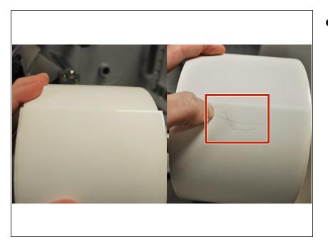
Direct transfer labels will show a grey mark if you scrape your thumbnail along it, while thermal transfer will not. Make sure the labels you are using are of the Direct Thermal variety.
