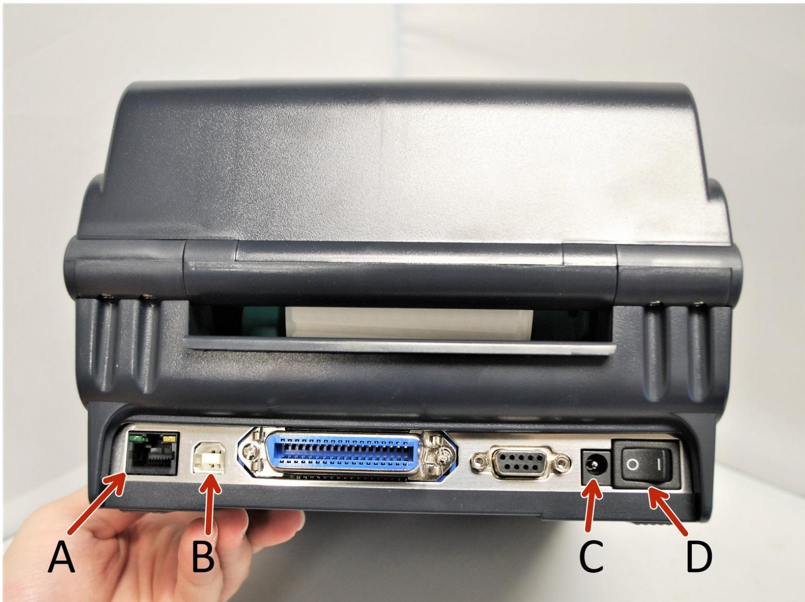
**Step 1 — Identifying the Printer's Rear Power Switch and Cable Ports**
